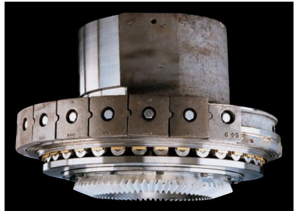
Due to the tighter tolerances of the wedge plate's roller bearing's —1/10 those of a bronze-bushing cone—a true setting is maintained. The tighter tolerances reduce oversize to about 20% instead of the 50% as with bronze-bushing cones when making a 1/2" (12.7 mm) minus product. This allows more feed material in the circuit with less recirculation and that means more production.
