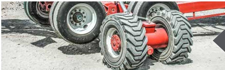
ENCLOSED DRIVE PROTECTS GEARING FROM DEBRIS
