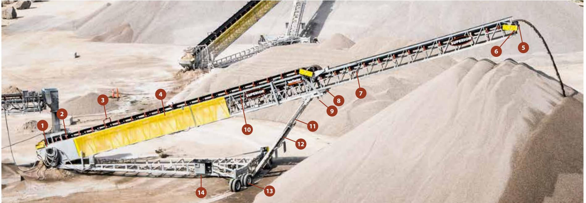
1/ **CHEVRON® PULLEY:** Patented v-shaped pulley deflects fugitive material to extend pulley life and lessen belt wear. In addition, constant belt contact reduces vibration and noise generation by 50 decibels.
