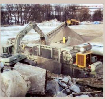
This Lippmann impactor is a brute of a crusher that handles concrete full of rebar, asphalt and other C&D debris to produce highly saleable materials.
