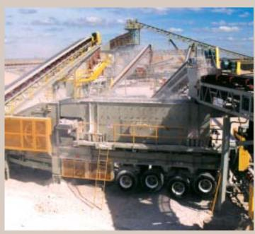
Lippmann designs and supplies primary and secondary impact crushing plants. The 5165LS shown above in this modern aggregate processing installation is a highly popular plant for secondary crushing applications.
