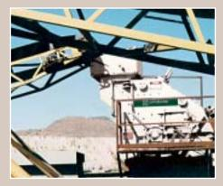
Feeding method is critical with an impact crusher. Optional feed chute designs are available to allow the impactor to be fed from three sides with a stacking conveyor.
