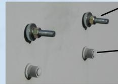
Clamp bar bolts w/ spherical washers
