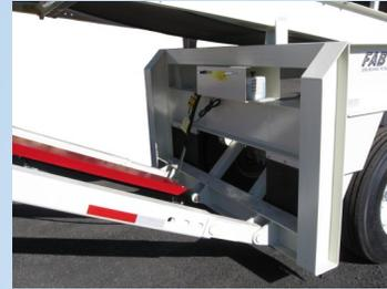
Hydraulic conveyor lift on Discharge conveyor.
