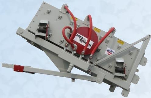
4 Bar Wash System with 7 spray nozzles per bar, 1 1/2" brass gate valves, water manifold with 3" inlet, and clean-up hose hook-up. (Requires 140 gpm at 40 psi water source)
