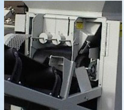
24"x5' belt feeder hopper has adjustable weighted feed gate.
